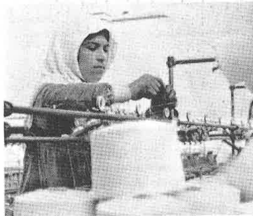
A woman worker prepares the automatic winding machine at the Shahnaze textile factory in Isfahan.
